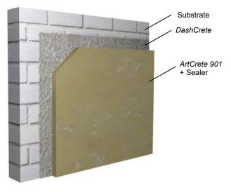
**SURFACE PREPARATION** • *ArtCrete 901* can be applied on an array of bases. It is very compatible with old concrete, masonry, and new concrete. All bases should be sufficiently rigid, clean of any surface contamination that may prevent good suction. Dense, smooth surfaces and those retaining excessive amount of form release agent can cause de-lamination of the plaster from the base.
